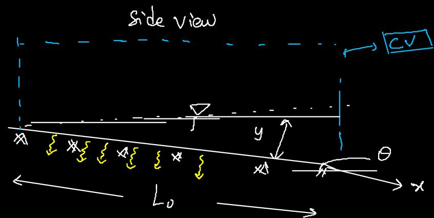
Ⓐ  $L_o$  = Length of ground below flow,  $V$  = outlet flow velocity.
