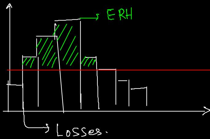
$\phi$ -Index → Constant rate of infiltration that would yield an ERH with a total depth equal to the depth of direct runoff ( $R_d$ )
