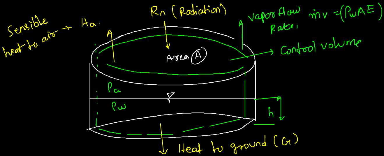
④  $\dot{m}_v = \text{Vapour flow Rate} = \underline{\underline{P_w A E}} \quad (E = \text{Evaporation rate})$
