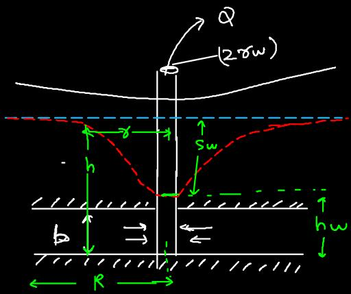
$$\begin{aligned} & \rightarrow v_r = \text{Radial velocity} \\ \Rightarrow v_r &= k \cdot \left( \frac{dh}{dr} \right), \quad \text{in cylinder of area} = (2\pi r) b \\ \Rightarrow \text{Discharge}, \quad Q &= v_r \cdot A \Rightarrow Q = (2\pi r) b \cdot k \cdot \frac{dh}{dr} \end{aligned}$$
