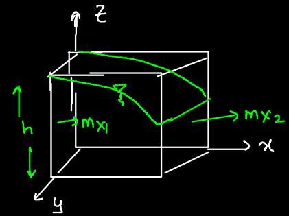
$$\Rightarrow \iint_{C.S} \beta P \vec{v} \cdot d\vec{A}, \quad \begin{array}{l} \text{X dirn:} \\ \text{---} \end{array} \boxed{m_{x1} = P v_x \cdot (h \Delta y)} \quad \left| \begin{array}{l} \text{mass influx} \\ \text{in } x \text{ dirn.} \\ m_{x1} \end{array} \right.$$
