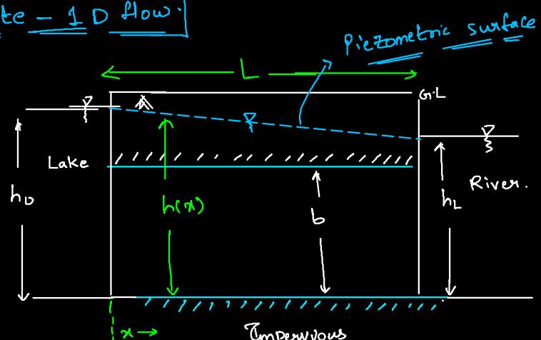
$$\Rightarrow \boxed{h = c_1x + c_2} \rightarrow \text{Find } c_1 \text{ and } c_2$$
