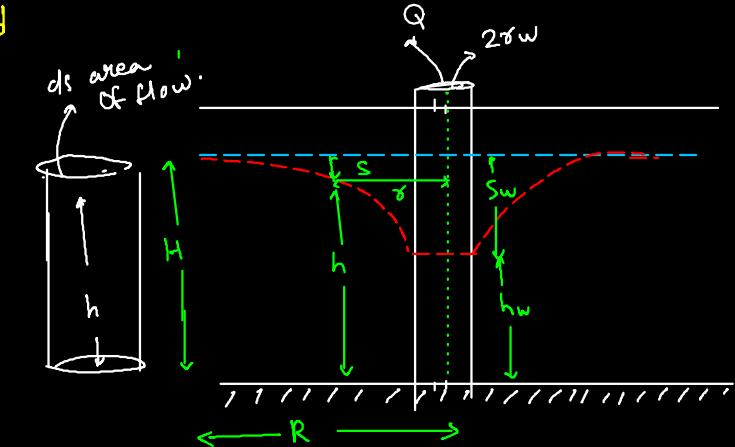
$$\int_{r_1}^{r_2} \frac{Q}{2\pi K} \frac{dh}{r} = \int_{h_1}^{h_2} h dh$$
